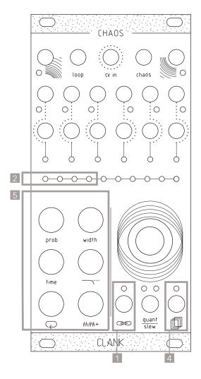
double tap on the *Input assign* button [1]. Now, each one of the *modifiers buttons* (plus *Ioop*) [5] corresponds, respectively, to each one of the six channels. (Ch.1 is Probability, Ch.2 is Width, Ch.3 is Time and so on..).
